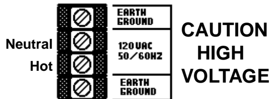
Figure 3E: AC Connections
