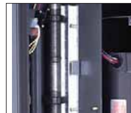
limit switches direct driven and easily adjustable
